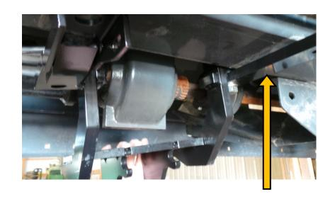
\*\*Make sure bars are flush to tubing before tightening
