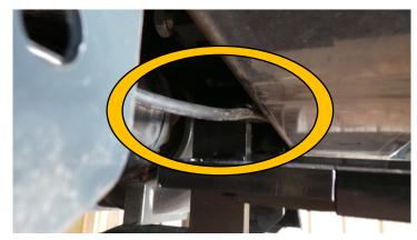
4. Bushings need to be in place when tightening supplied bolts (reuse existing washers)
