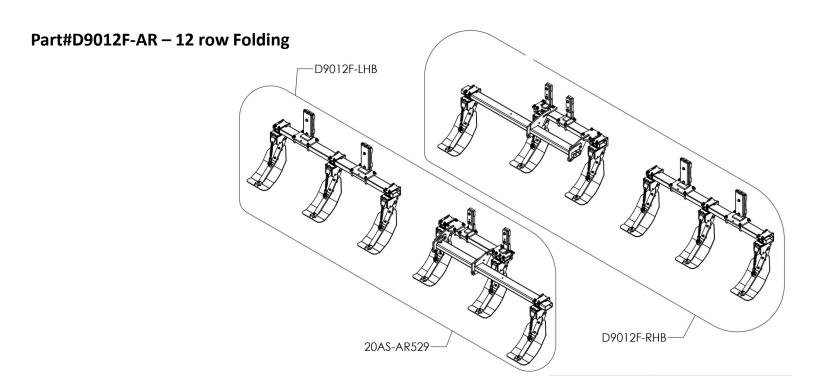
Step 1. Do Not Tighten Bolts or Nuts
