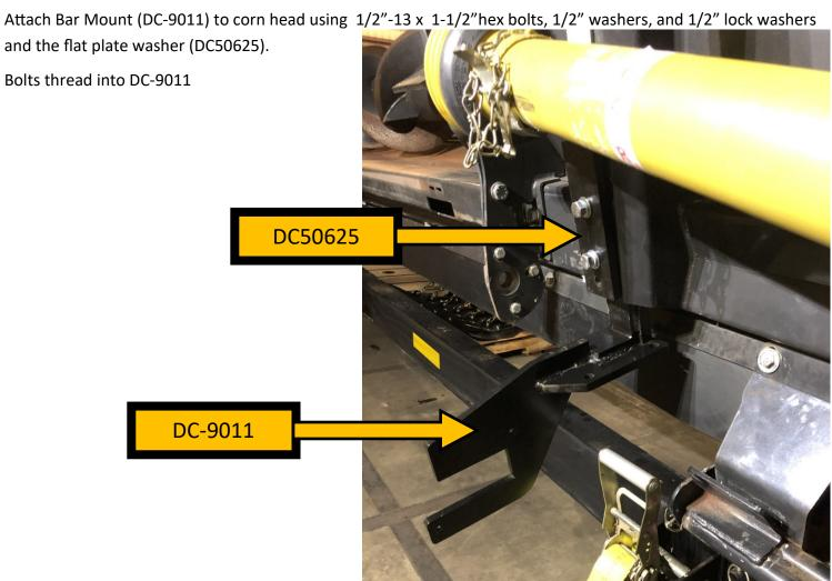
Step 4. Do Not Tighten Bolts or Nuts
