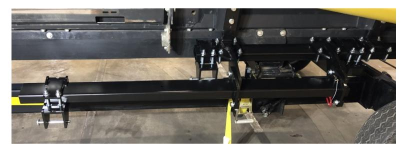
Step 9. Do Not Tighten Bolts or Nuts
