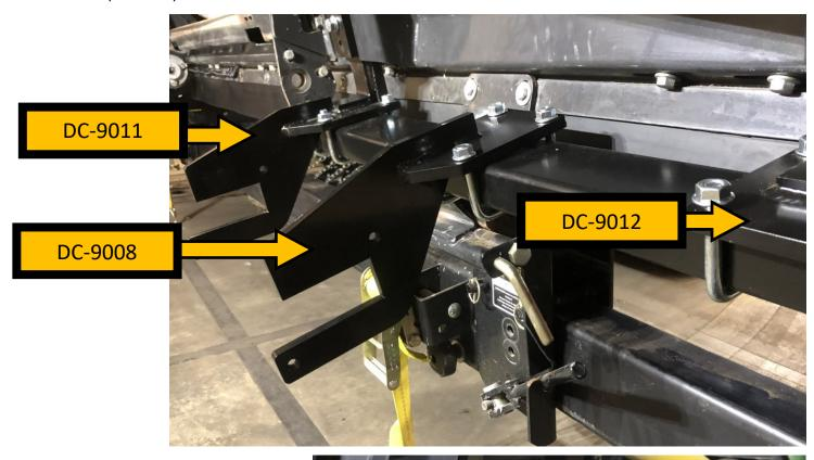
Step 8. Do Not Tighten Bolts or Nuts
