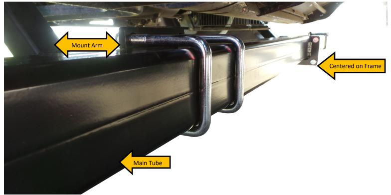
$\begin{tabular}{ll} Step 4. \\ Attach extension arms to main tubes on both sides using u-bolts and nuts. \\ \end{tabular}$
