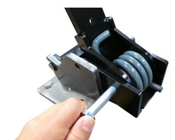
\*The easiest way to compress the shoe is to place it into the mount on the corn head and use that for leverage\*
