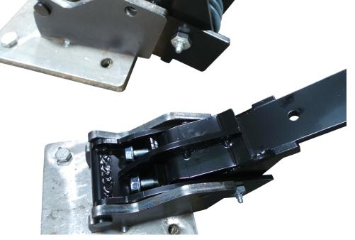
Keep shoe compressed and bolt stop into 3 position arm
