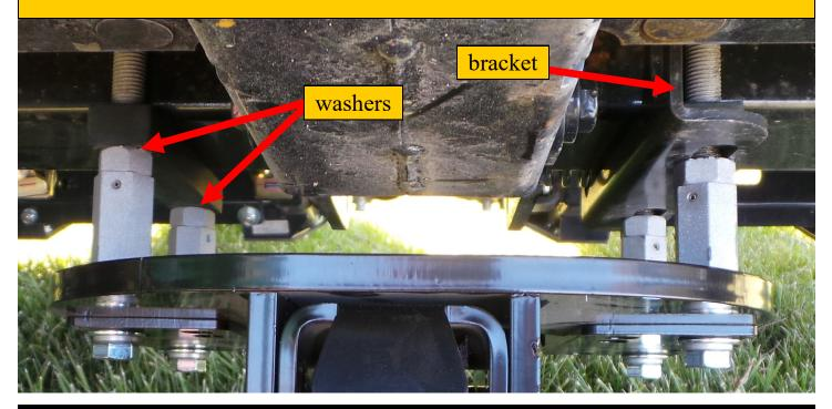
For ease of installation, before removing existing gearbox bolts, place a clamp on this side of bracket to keep spring compressed.
